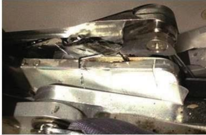
Figure 25 – A mobile phone crushed in an electrically adjustable seat
