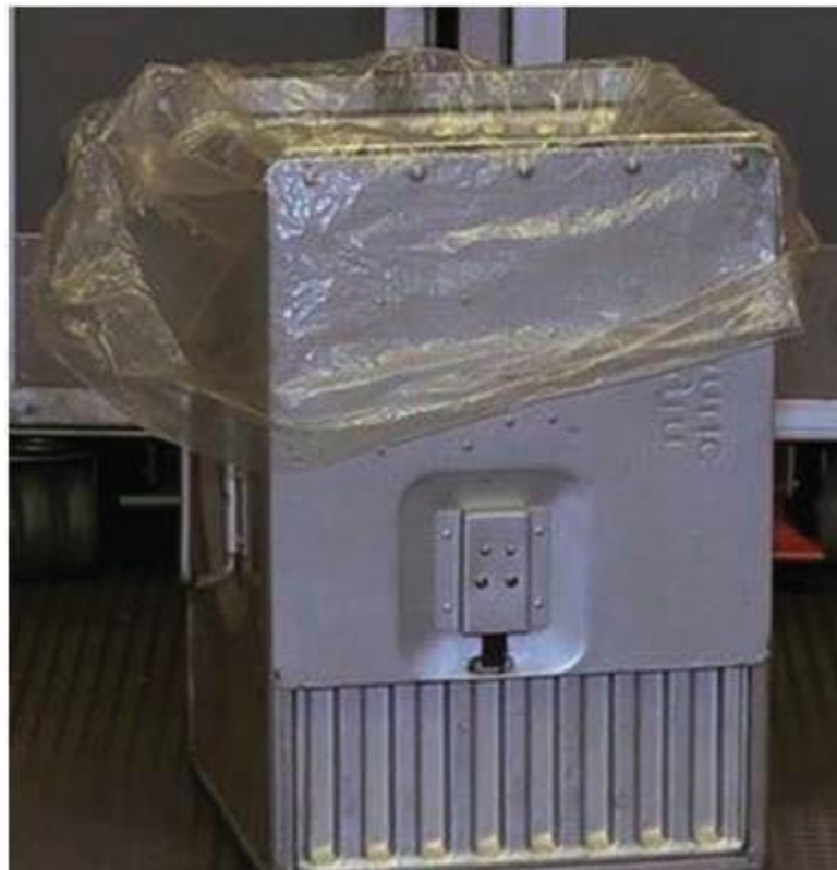
Figure 24 – A bar box made watertight by using a plastic bin liner
