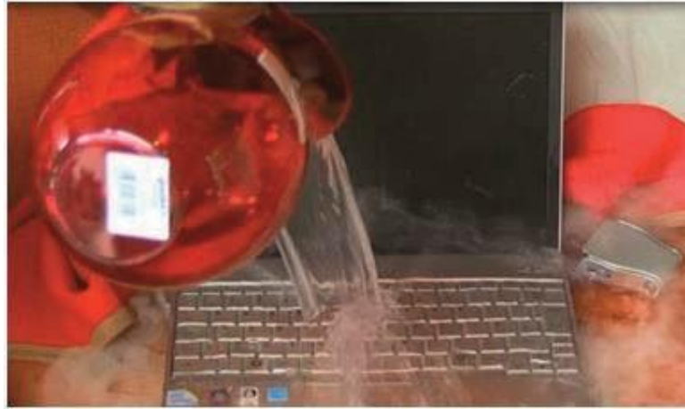
Figure 19 – A laptop being doused with water from the galley
