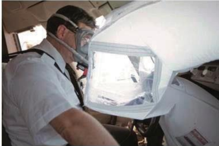
Figure 13 – Smoke displacement system (EVAS – Enhanced vision assurance system)
