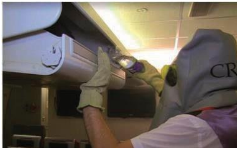
Figure 20 – Applying water to a burning device without removing it from the overhead locker. It is important to note that liquid may turn to steam when it is applied to heated batteries
