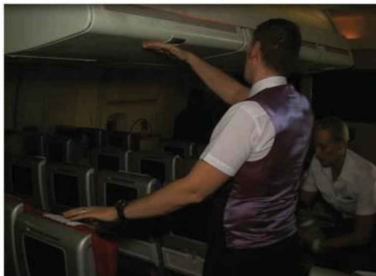
Figure 17 – Determining the location of a fire in an overhead locker
