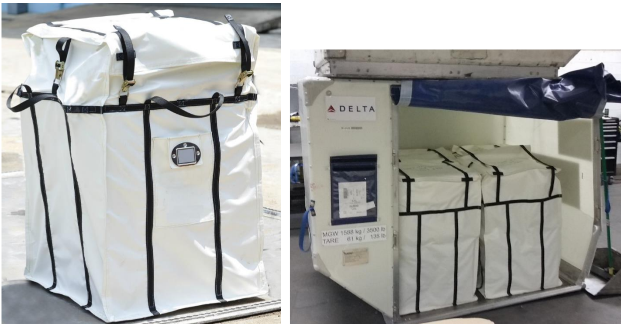
Figure 12 – Fire containment bags loaded on a certified aircraft pallet and in a certified lower deck aircraft container
