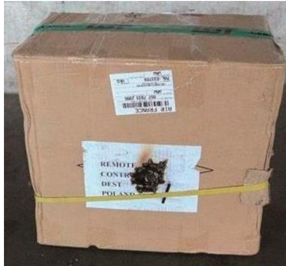
Figure 4 – Fire damage to a package of incorrectly packed lithium metal button cells, which occurred after unloading
