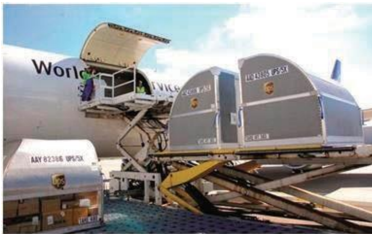
Figure 10 – Main deck fire-resistant containers
