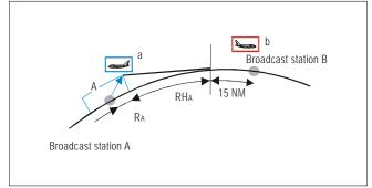
Separation distance between two stations providing aeronautical broadcast services; max range is 200 NM
