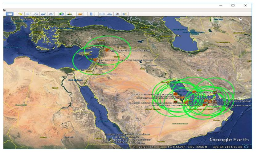
VOR/DME - No frequency on 100 kHz channels could be assigned to 17 VOR/DME facilities
