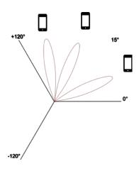
AAS antennas only radiate in a single beam at a time but switch from beam to beam very quickly. This means that the more mobiles there are in one direction, the higher power radiated in that direction!
