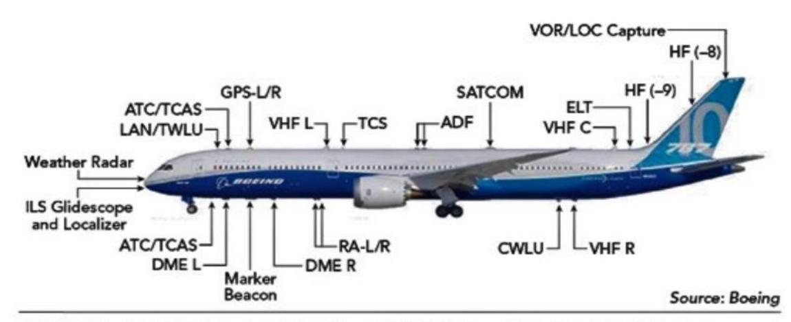
LAN/TWLU - Terminal Wireless Local Area Network (LAN) Unit ATC/TCAS - Air Traffic Control/Traffic Collision and Avoidance System DME - Distance Measuring Equipment RA - Radio Altimeter GPS - Global Positioning System TCS - Terminal Cellular System ADF - Automatic Direction Finder CWLU - Crew Wireless LAN Unit ELT - Emergency Locator Transmitter HF - High Frequency Radio VOR VHF - Omnidirectional Ranging
