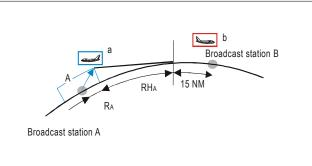
Separation distance between two stations providing aeronautical broadcast services; max range is 200 NM
