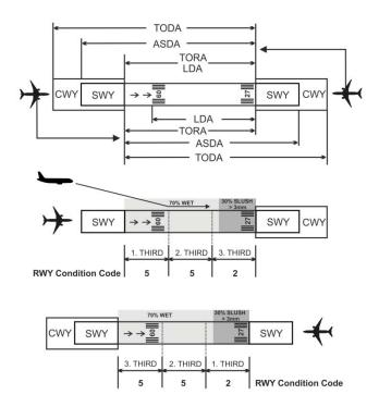
Figure 2. Reporting of runway condition code for runway thirds from ATS to flight crew on a runway with displaced threshold
