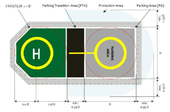
Figure 14-1 1D FATO/TLOF with associated 1D parking area (separated by a parking transition area
