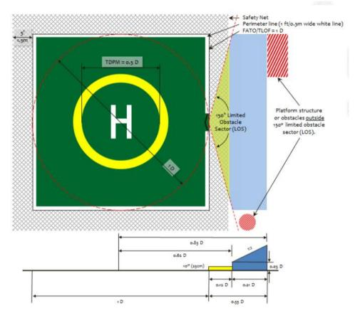
Figure 10-6 Square obstacle limitation sectors and surfaces for 1D FATO and coincidental TLOF
