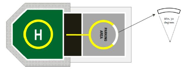
Figure 14-7 Touchdown Parking Circle and Parking Circle Orientation Marking (PCOM)
