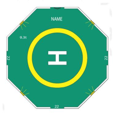
Figure 13-1 Typical floodlighting arrangement for an octagonal helideck
