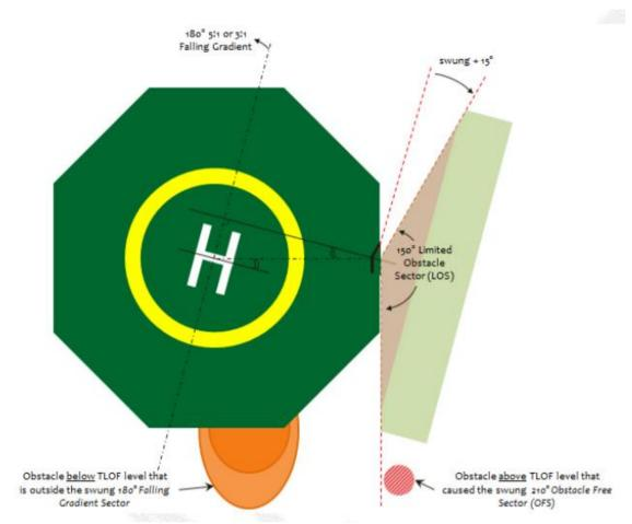
Figure 12-1 Helideck identification marking reflecting a swung obstacle free sector (in this case the OFS is swung by 15 degrees in a clockwise direction to avoid an obstacle)
