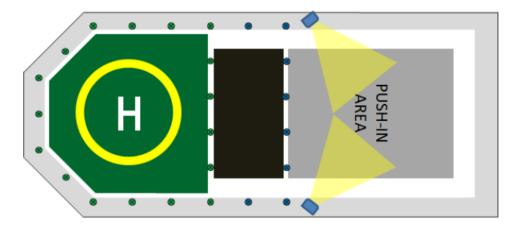
Note — The Push-in Area shall be provided with flood lighting. If hover taxi and/or ground taxi is still allowed in the Transition Area, the TA perimeter lights should be in a blue colour. If no taxi-ing is allowed in the TA, then flood lights would also be recommended
