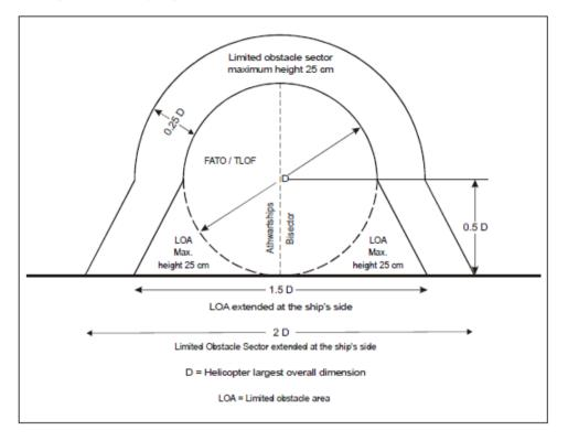
Figure 10-9 Ships-side non-purpose-built helideck obstacle limitation sectors and surfaces
