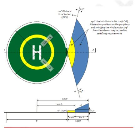
Figure 10-4 Circular obstacle limitation sectors and surfaces for 1D FATO and coincidental TLOF
