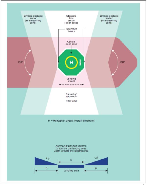
Figure 10-8 Amid-ship location – Shipboard helideck obstacle limitation surfaces
