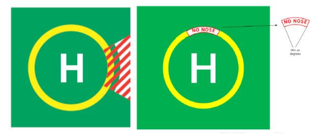
b) The sector of the TD/PM circle, opposite from the personnel access point, should be bordered in red with the words "No Nose" clearly marked in red on a white background as shown in Figure 12-9. When positioning over the touchdown/positioning marking circle, helicopters should be manoeuvred so as to keep the aircraft nose clear of the "No Nose" marked sector of the TDPM circle at all times. The minimum prohibited "NO NOSE" marking should cover an arc of at least 30 degrees.
