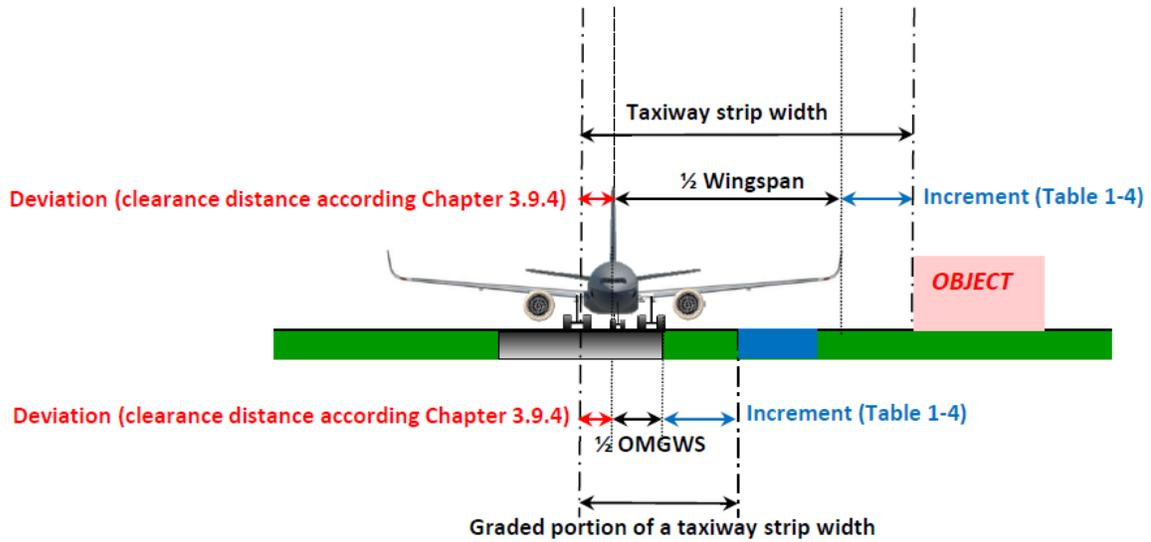
Graded portion of a taxiway strip in relation to taxiway to object distance according to Table 3-1 .
