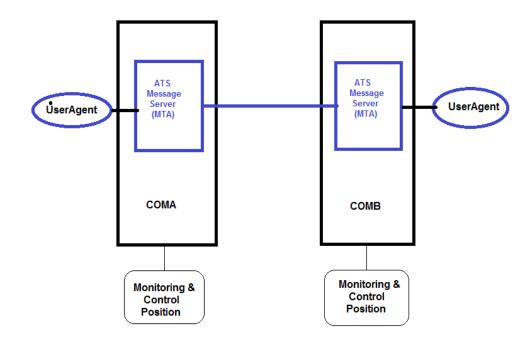
The test can be performed in AMHS Network and unnecessary to have direct AMHS link between the two COM centers, the traffic can be exchanged via intermediary(ies) COM center(s), which should be involved in the test activities.
