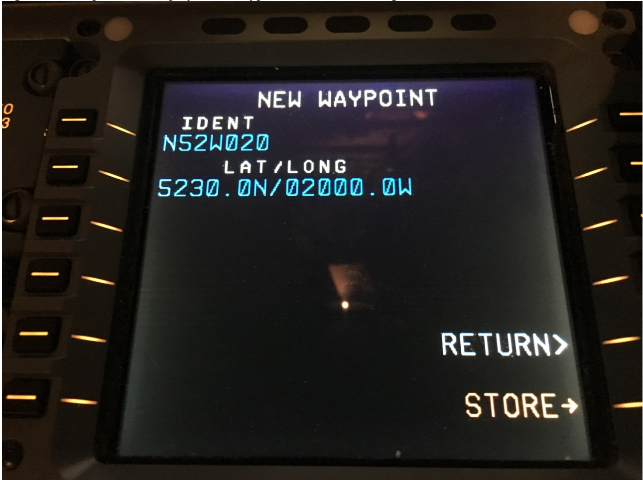
Figure 1 Example FMC Display: Full Waypoint Latitude and Longitude (13-characters) inserted into FMC
