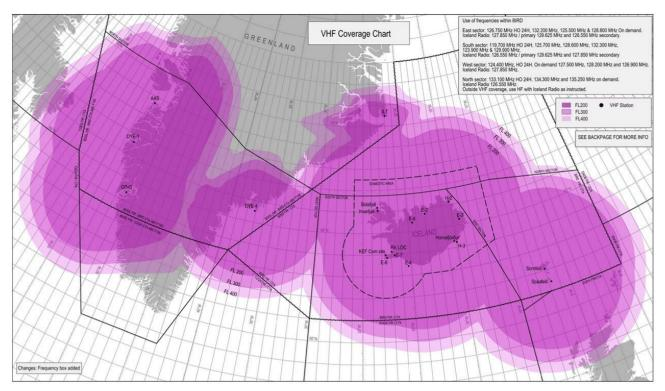
Figure 6-1 Reykjavik Control Direct Controller Pilot VHF Coverage
