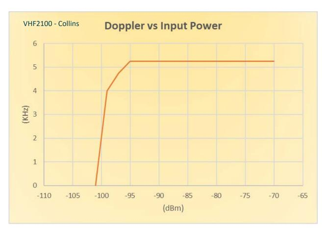
Maximum Doppler shift at the receiver input for which the VDL2 link is established
