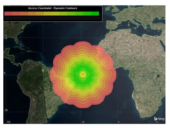
ADS-B - Aircraft to Satellite (Rx) Coverage (S/N, Detectability, Antenna ....)
