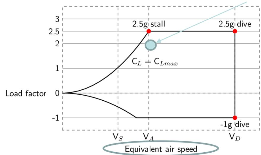
Problem is that we have mutated the V-n diagram to use indicated airspeed, and we have not accounted for compressible (Mach) effects
