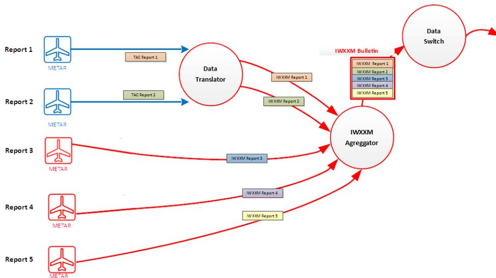
Figure 4: Aggregation of TAC and IWXXM data
