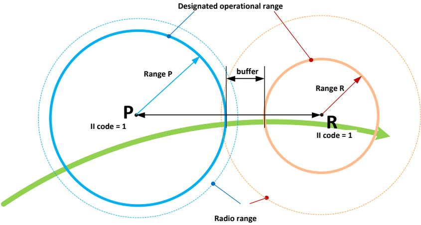
Figure 10. – Minimum separation distance between interrogators having the same II code
