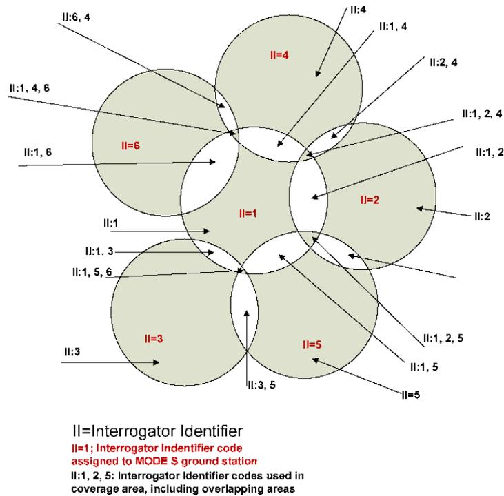
Figure 9. – Example of II code assignments
