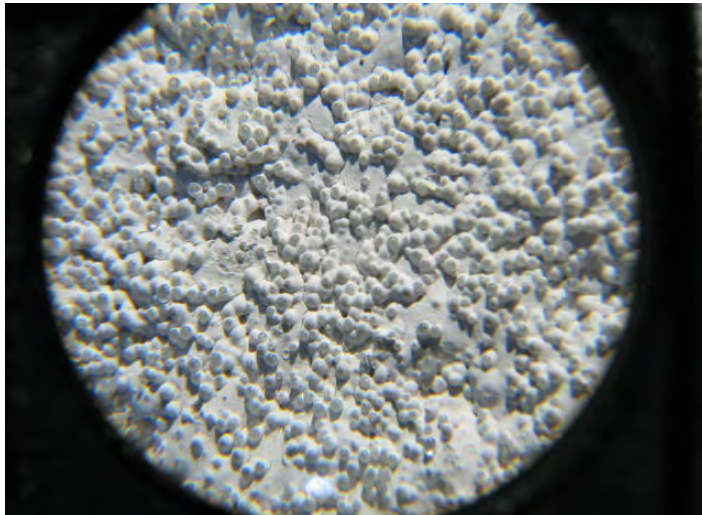
FIGURE 6-64. EXCESSIVE WICKING OF PAINT OVER BEADS.
