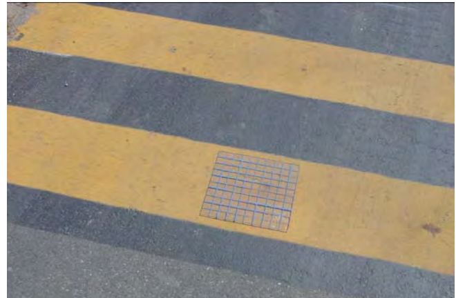
FIGURE 6-74. GRID FOR COMPLIANCE WITH DEGREE OF PAINT REMOVAL.
