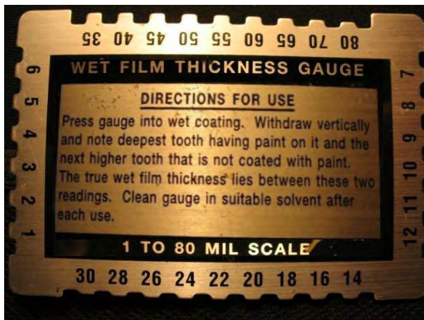
FIGURE 6-61. WET FILM GAUGE.
