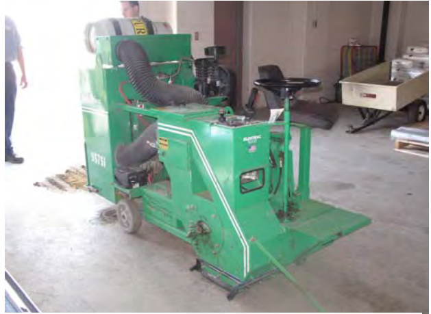
FIGURE 5-13. SHOTBLASTER WITH A 10-INCH CUT.
