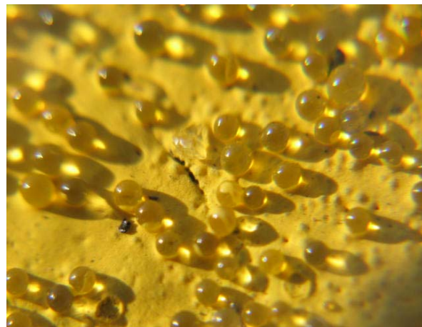
FIGURE 3-11. POOR TYPE IV BEAD EMBEDMENT.
