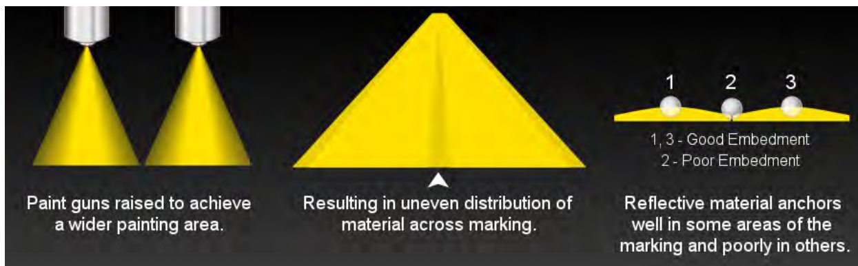
FIGURE 6-48. IRREGULAR FILM THICKNESS ACROSS THE LINE PERFORMS POORLY.
