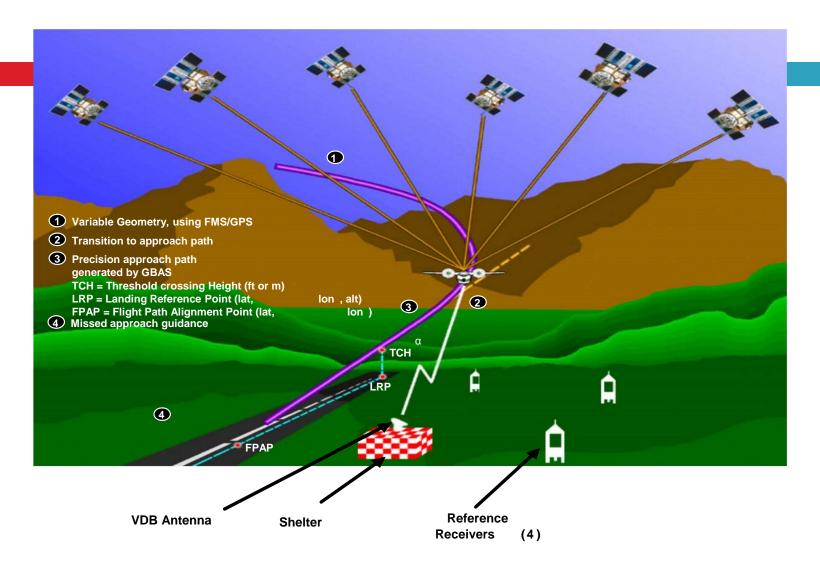
**PILOT PROJECT** AT CHENNAI **SMARTPATH EQUIPMENT** ALLOW TO **DESIGN** OF 26 APPROACHES INCLUDING **CURVED PATH** APPROACHES WHICH WILL HELP IN KEEPING FLIGHT CLEAR OF NOISE SENSITIVE ZONES
