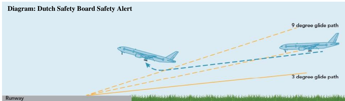
Figure 2: Sudden pitch up commanded by the autopilot system due to the signal reversal above the 9 degree glide path
