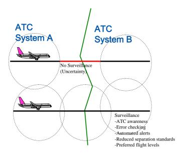
Surveillance data allows differences to be identified early before they become a problem. It allows the application of automated safety net tools that automatically alert controllers to a range of problems such as aircraft at the wrong flight level.
