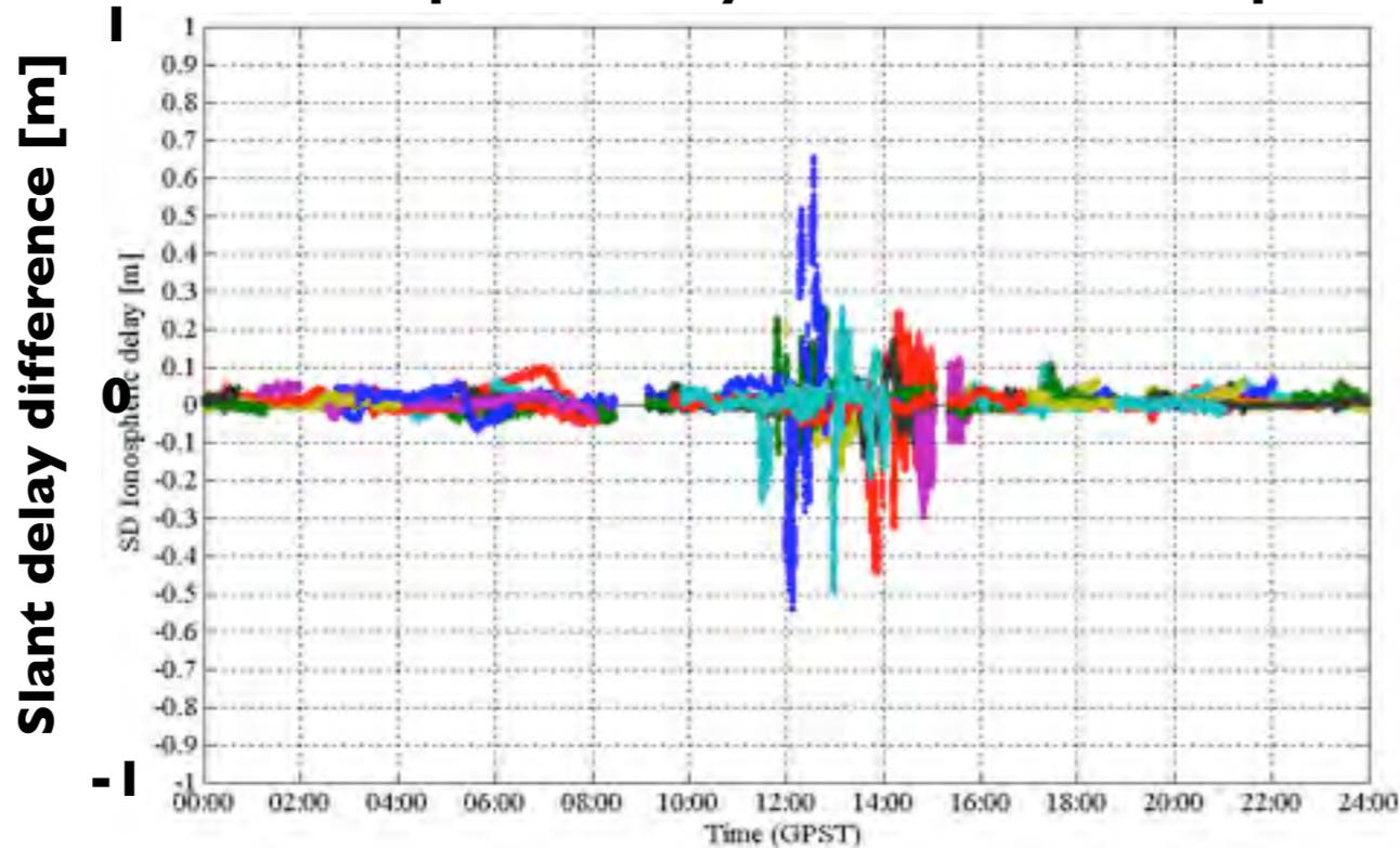
Ionospheric delay difference (single difference) between two GEONET stations separated by 6.3 km
