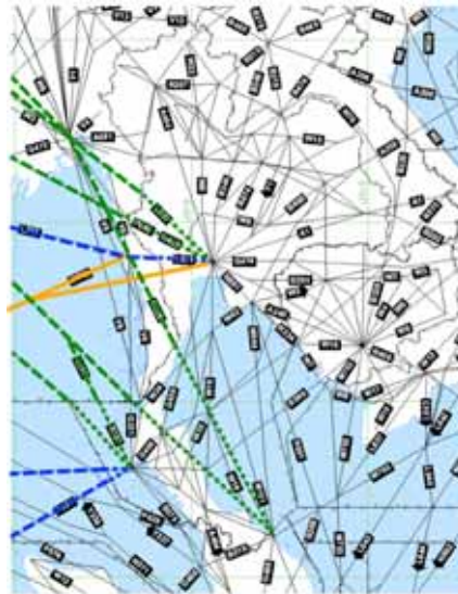
Figure 1: Proposed Routes for inclusion in Phase 2 Reduced Horizontal Separation Implementation Note: Orange Routes: Phase 1 RHS Green Routes: AR 4 Major Traffic Flow Proposed Routes for Phase 2 RHS Blue Routes: AR 10 Major Traffic Flow Proposed Routes for Phase 2 RHS
