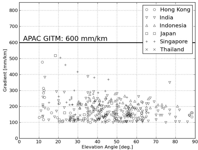
Figure 1. Ionospheric gradients (greater than 100 mm/km) observed in the APAC region and adopted upper bound of the gradient as a function of satellite elevation angle.
