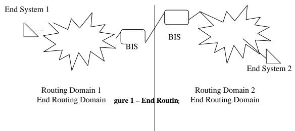
A transit routing domain routes PDUs between two or more routing domains, and may as an option also act as an end routing domain. An example of a transit domain is where a set of backbone routers is configured in their own routing domain with all of the end systems in end routing domains attached to the backbone.
