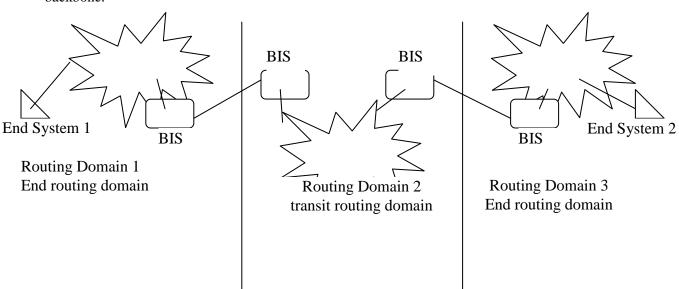
Note: A transit routing domain may or may not be part of the backbone. That is, a routing domain may consist of BISs none of which are backbone routers.
