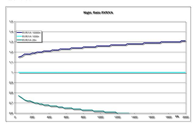
When visibility is considered to be VA, the ratio between RVR and VA is much lower than when considering MOR.
