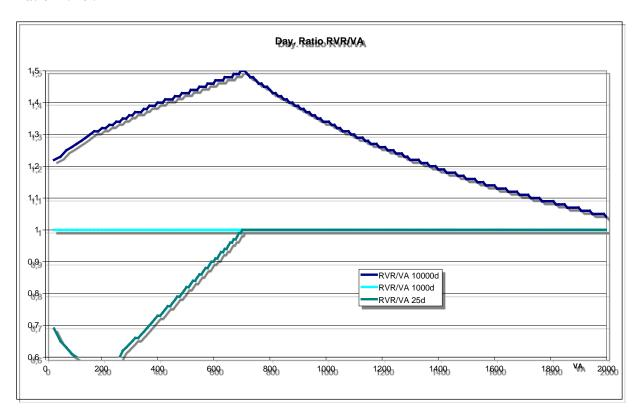
When visibility is considered to be VA, in day conditions and HI lighting, the ratio between RVR and VA increases up to 1.5 and then decreases down to 1. This curve shape is due to the respective influence of lighting intensity in the calculation of RVR and VA.
