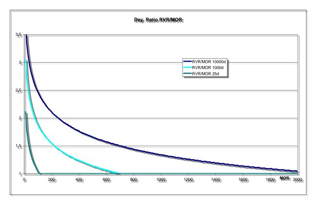
In day conditions and HI lighting, the ratio between RVR and MOR decreases from 2 down to 1. For low intensity lighting, the ratio between RVR and MOR is 1 for any MOR values > 100m.
