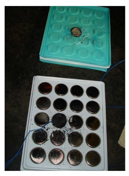
FIGURE 3: CELLS REMOVED FROM TRAYS, SHORT-CIRCUITED, AND OBSERVED
