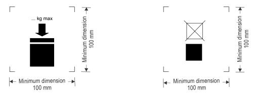
$_{\neq}$  Figure 6-1. IBCs capable of being stacked Figure 6-2. IBCs not capable of being stacked
