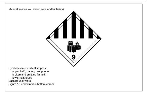
Figure 5-26. Miscellaneous dangerous goods — lithium batteries, Class 9
