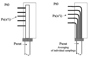
Multi-hole mixing probe (Mixing in the probe) Mixin
