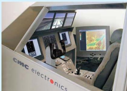
**A dynamic test bed provides avionics systems integrators with important flexibility while eliminating the costly and time-consuming need to use actual hardware in building a replica of an aircraft's avionics suite.**
