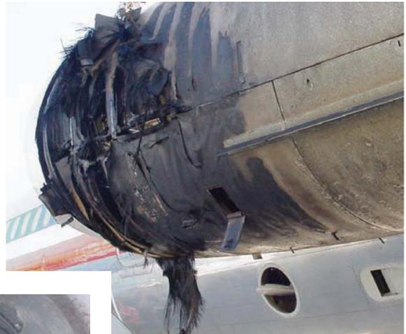
**Wildlife strikes, the vast majority of which involve birds, cost airlines about \$500 million per year in the U.S. alone. Above: An uncontained engine failure and fire occurred after a cormorant was ingested into this MD-80's port engine in September 2004. Left: Engine damage resulting from collision with two Canada geese in September 2003; one fan blade separated from the disk and penetrated the fuselage.**
