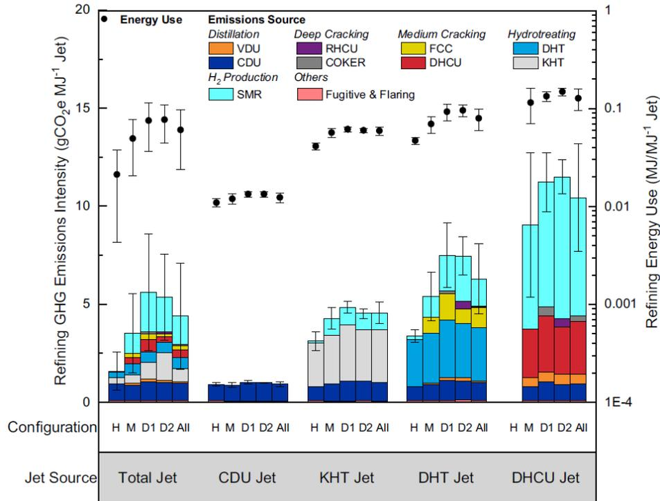
DHT Jet = prod. from diesel hydrotreater    DHCU Jet = prod. from distillate hydrocracking unit
