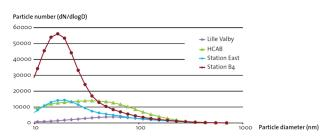
Figure 2. Particle number measurement results at Copenhagen Airport. Measurements for an urban busy street (HCAB) and rural background (Lille Valby) are shown for comparison.
