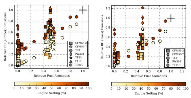
Figure 2. Measured normalized black carbon (BC) number and mass emissions as a function of normalized aromatic content and engine setting (Speth et al., 2014).
