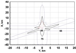
**Figure 4**. Noise Contours Predicted By Means of the Improved Calculation Method.
