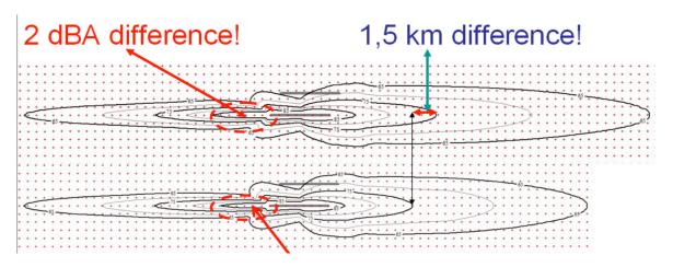
**Figure 8b.** IsoBellaResults for B-737-400Noise Contours (approach/landing and take-off/climbing) are Higher When Using Input Data for Flight Parameters Observed in Operations; and Lower for Balanced Input Data for Flight Parameters
