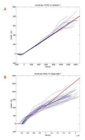
**Figure 6.** Flight Profiles (Height Via Distance) Observed In Operation (blue lines) In Comparison With Balanced Prediction (red lines): A – Arrival; B – Departure.<sup>10</sup>
