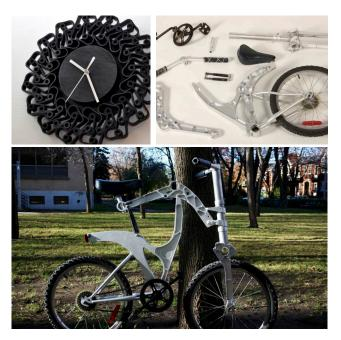
Figure 4. Re-designed leftover aircraft material
