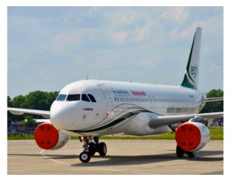
**Figure 2.** An aircraft with an e-taxi system installed taxiing using only the power from the APU. Source: http://articles.sae.org/12662/
