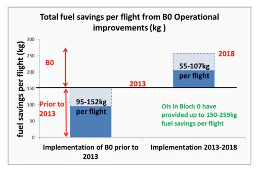
Figure 5. Range of ASBU Block 0 per-flight Fuel Savings
