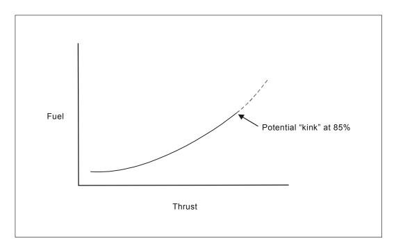
Figure 3-A1-2. Diagrammatic illustration of twin quadratic curve fit
