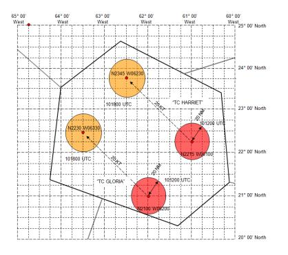
YUDD SIGMET 2 VALID 101200/101800 YUSO – YUDD SHANLON FIR/UIR TC GLORIA FCST AT 1200Z N2100 W06200 CB TOP FL500 WI 20NM OF CENTRE MOV NW 20KT WKN FCST 1800Z TC CENTRE N2230 W06330 AND *TC HARRIET FCST AT 1200Z N2215 W06100 CB TOP FL400 WI 20NM OF CENTRE MOV NW 20KT WKN FCST 1800Z TC CENTRE N2345 W06230*=
