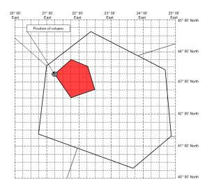
YUDD SIGMET 2 VALID 101200/101600 YUSO – YUDD SHANLON FIR/UIR VA ERUPTION MT ASHVAL PSN N4315 E02115 VA CLD OBS AT 1200Z WI N4315 E02145 – N4345 E02145 - N4230 E02215 – N4245 E02230 – N4230 E02145 -N4315 E02115 FL250/370 MOV ESE 20KT NC=
