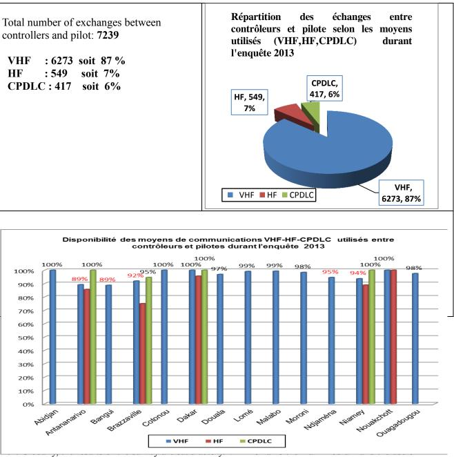
CPDLC is increasing in all the FIRs (increasing of airlines equipped); The use of HF is decreasing but still remains the only mean used in both desert and ocean in the centers not yet equipped CPDLC.
