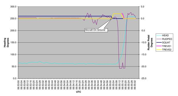
HEADING vs RUDDER PEDAL POSITION SQUAT SWITCH vs THRUST REVERSERS
