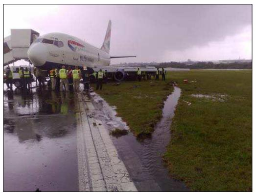
Figure 4. Shows the final position of the aircraft as it came to rest
