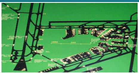
GROUND MOVEMENT RADAR – USED BY ATC AS PART OF ASMGC TO MONITOR NOT ONLY AIRCRAFT ON THE GROUND, BUT ALSO OPERATIONAL VEHICLES
