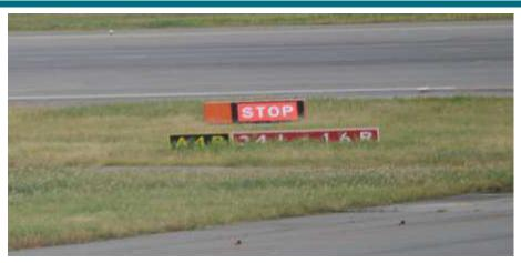
ENHANCED VARIABLE MESSAGE SIGNAGE AT RUNWAY HOLDING POINT TRIALLED BY JAPANESE CAA AT TOKYO NARITA TO STRENGTHEN EXISTING RUNWAY INCURSION PREVENTION MEASURES – SIGN SHOWING "STOP"
