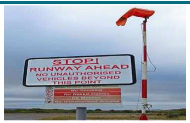
A VARIATION SIGN USING STOP WITHOUT INSTRUCTION – BUT WITH WARNING USED AT AN AIRFIELD WITH VEHICLE RUNWAY ACCESS BUT NO ATC
