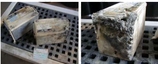
Batteries were packaged together in same box. Package caught fire in air cargo sort facility.
