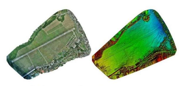
Figure 1: Orthomosaic and the corresponding sparse Digital Surface Model (DSM) before densification. Figure 4: Orthomosaic and Digital Surface Model
