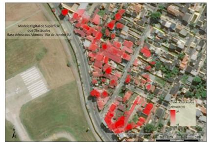
Figure 9: Digital surface model of obstacles located in the approach area of threshold 29 of the Campo Délio Jardim de Mattos (SBAF) aerodrome
