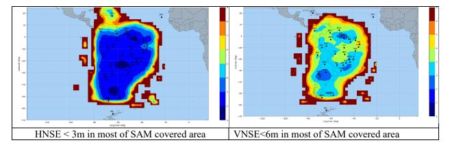
2.14 Measured position accuracy performances remain very efficient and fully compatible with APV-I vertical guidance approaches.
