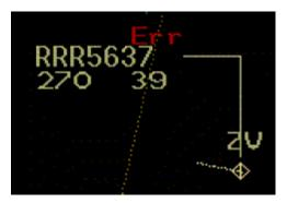
Err: Transmission failed, interface in failed state
