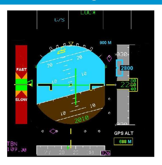
BUSS option replaces the normal PFD speed- and altitude tapes with AOA and GPS ALT when all ADRs are switched OFF.
