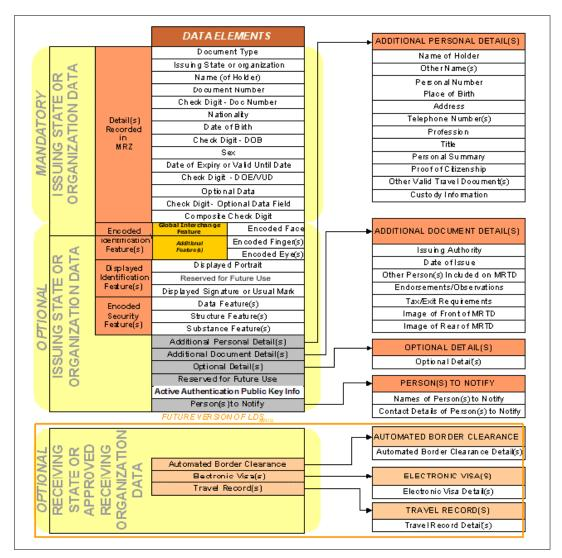
Figure 8. Mandatory and optional elements of the Logical Data Structure
