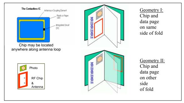
Figure 5. E-passport configurations
