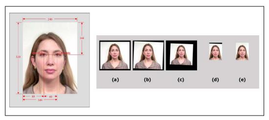
Figure 7. Illustration of the steps in the creation of a Token Frontal Image
