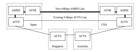
NOTE: The domestic service can be either AFTN or AMHS, or both. (Gateway function is necessary for domestic AFTN Service.)
