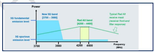
**Source:** RTCA Paper No. 274-20/PMC-2073 – (Figure 3-1: Spectrum Illustration Showing 5G Fundamental and Spurious Emissions, page 20).
