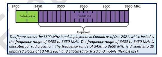
• Maximum power is 68 dBm/5 MHz up to 305 metres and 61 dBm/MHz for channel bandwidth less than 5 MHz Antenna above 305 m need to calculate the maximum power emission
