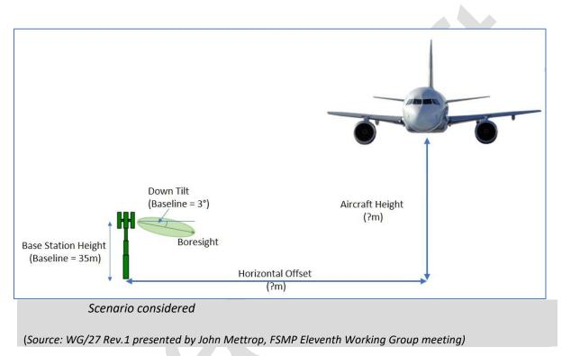
• For each angle during the approach of an aircraft, the required separation distance is calculated using the following ITU formula assuming free space path loss:
